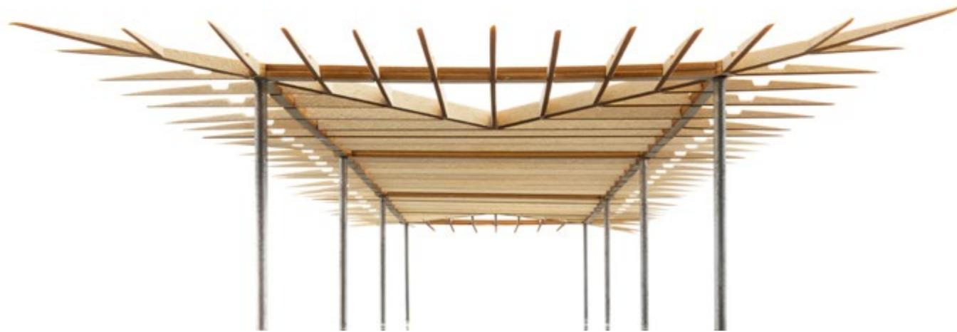
Conceived as a single element to provide shading beside the old port in Marseille, the detailing of this canopy is minimal. The perimeter is a single thin line, with the gutter set back inside the roof, with the canopy structure orientated to avoid an edge beam. Lateral stability is provided through frame action of the columns, which are fixed both at roof level and by the ground beams that connect the column bases.
