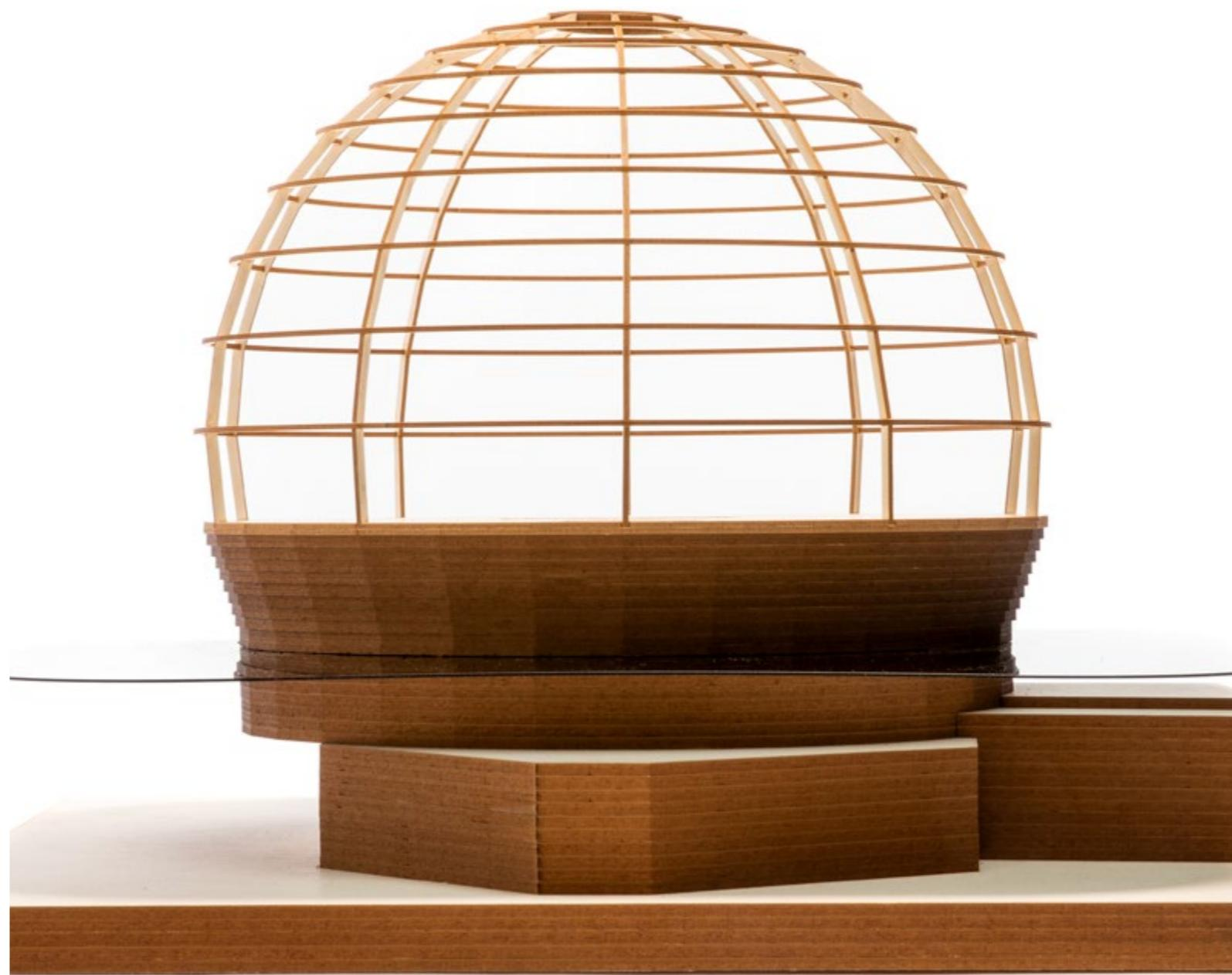
One of the unique features of this 30 metre dome structure is the structural interaction between the steel ribs and the glass panels. The glass panels provide bracing against buckling to the steel members, as well as stiffening the entire enclosure against lateral loads. The resulting steel structure is exceptionally small, with the ribs dimensioned at less than 1/200 of the dome span.
