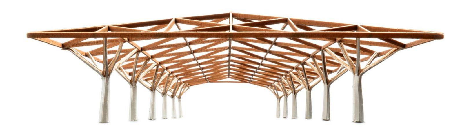
The roof structure of the new winery spans the 28 metres across the central space with a grid of beams that are three times shallower than what would be achieved with a classic beam system. The roof uses the pitched geometry to resist the applied loads through compression as well as bending. The supporting 'tree' structures provide both the vertical and lateral support to the roof.
