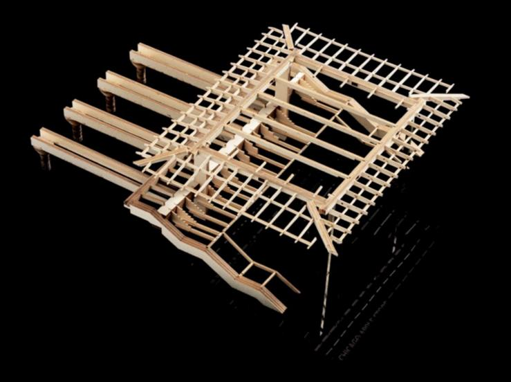
The central space is covered by a thin tapering roof that cantilevers approximately eight metres beyond the façade on each of the four sides. This structure is supported on only four steel columns to minimise the structure, while a mezzanine balcony cantilevers into the generous interior.
